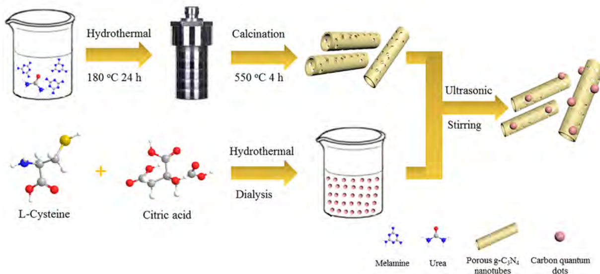
Scheme 1. Schematic illustration of the preparation for modified carbon quantum dots loaded hollow tubular carbon nitride (HTCN-C) samples.
