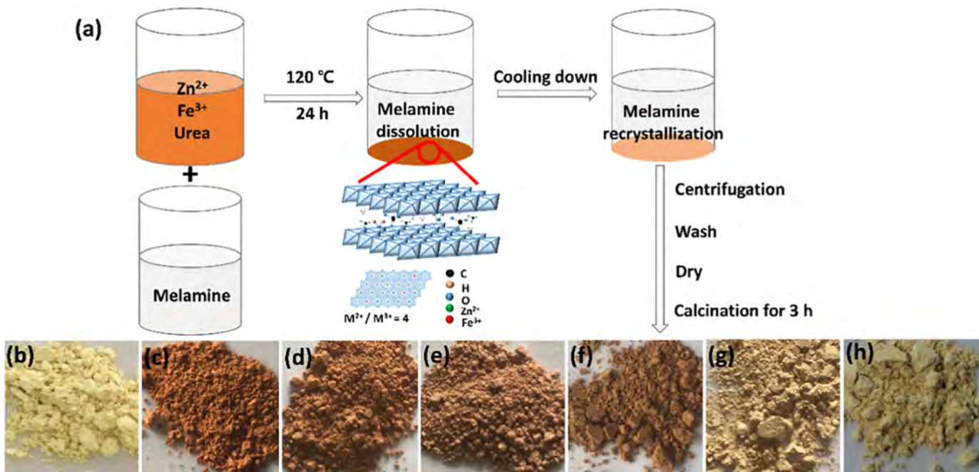
Fig. 6. (a) Schematic illustration of synthesizing the calcined Zn-Fe-LDH/g-C 3 N 4 composites; photographs of the g-C 3 N 4 (b), the calcined Zn-Fe-LDH (c), and the calcined Zn-Fe-LDH/g-C 3 N 4 products with different weight percentages of g-C 3 N 4 (d-h, from left to right: 0.5, 1.0, 5.0, 70, and 90 wt%). Reproduced with permission from ref. [97]. Copyright 2018 Elsevier.
