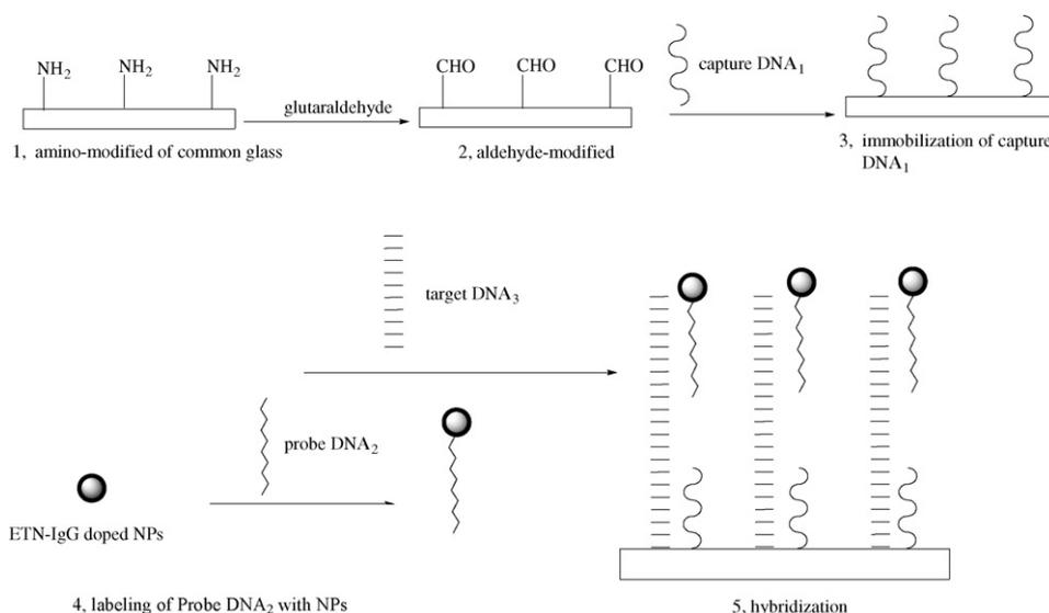
Fig. 1. The two-probe tandem DNA hybridization assay.
