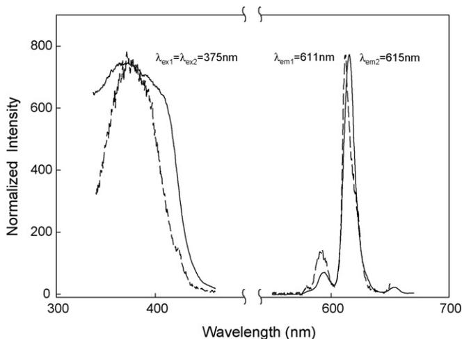
Fig. 4. Time-resolved fluorescence spectra for the ETN (—) and ETN-IgG doped NPs (---). For time-resolved spectra: delay time, 0.1 ms, gate time, 1.0 ms.
