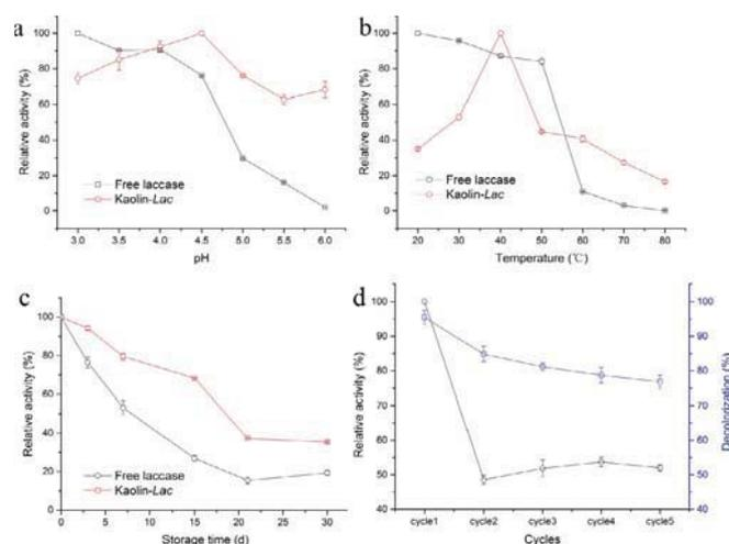
**Fig. 5.** a) pH stability of free laccase and Kaolin-Lac; b) Thermal stability studies of free laccase and Kaolin-Lac at 20–80 °C up to 120 min; c) Storage stability of free laccase and Kaolin-Lac; d) Operational stability of Kaolin-Lac and reusability of Kaolin-Lac for MG with the coexistence of Cd (II) decolorization.
