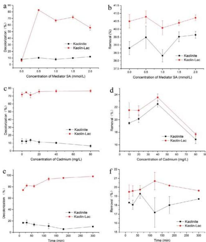
**Fig. 6.** a)&b) Effect of concentration of mediator SA on treatment of MG effluent mixing with Cd (II) by Kaolin-Lac; c)&d) Effect of concentration of cadmium on treatment of MG effluent mixing with Cd (II) by Kaolin-Lac; e)&f) Effect of time on removal rates of MG effluent mixing with Cd (II) by Kaolin-Lac.
