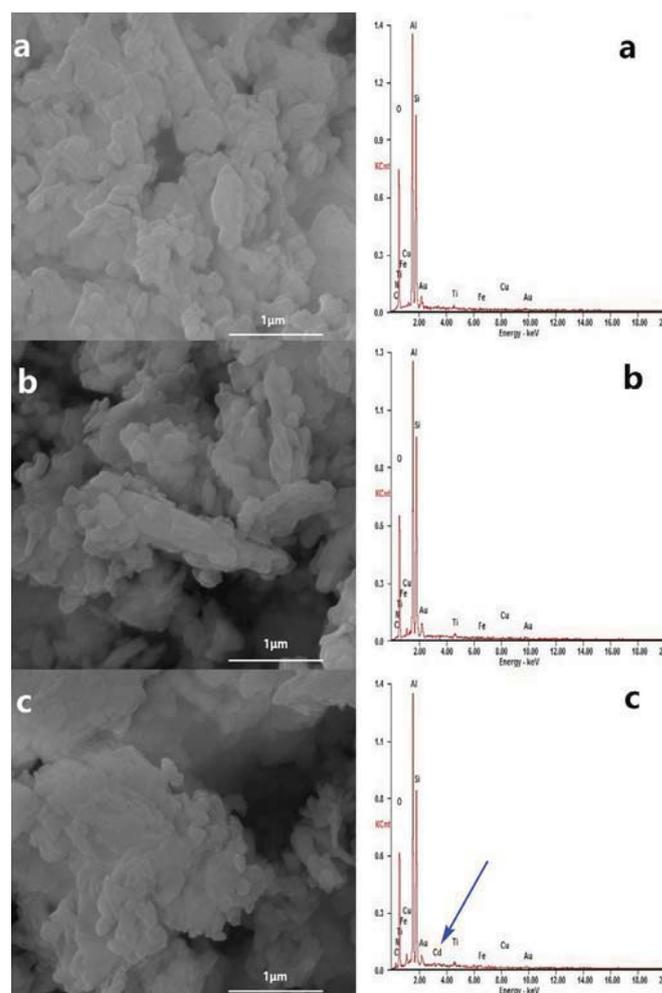
Fig. 2. SEM images and relevant EDS of the a) kaolinite, b) Kaolin-Lac, c) Kaolin-Lac after treatment.
