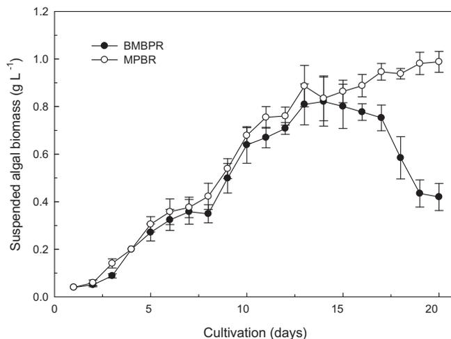
Fig. 2. The suspended algal biomass as a function of culture time in the reactors of biofilm membrane photobioreactor (BMPBR) and membrane photobioreactor (MPBR). The data are mean  $\pm$  standard deviation of three independent experiments.
