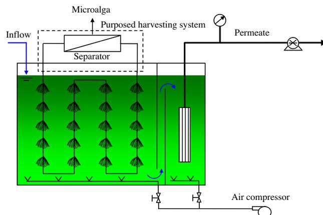
Fig. 1. Schematic diagram of the lab-scale biofilm membrane photobioreactor (BMPBR).
