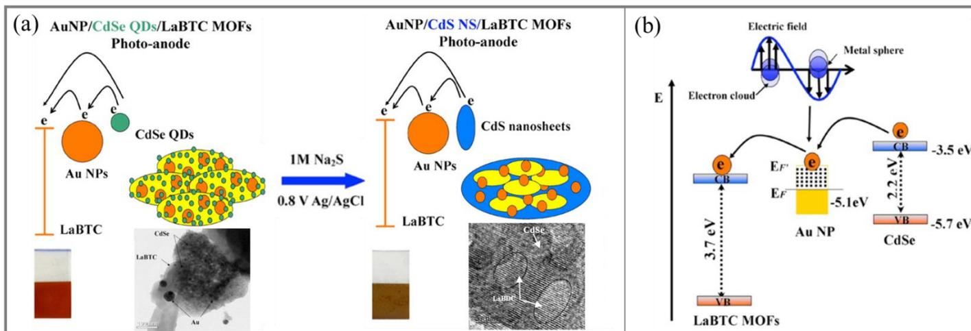
Fig. 7 (a) The schematic diagram of photoelectrode transformation from Au NPs/CdSe/LaBTC to Au NPs/CdS/LaBTC and the electron transport path of them. (b) The band energy diagram and electron transfer mechanism of Au NPs-CdSe QDs sensitized LaBTC MOFs. Reproduced with permission from ref. [13]. Copyright 2016 American Chemical Society.
