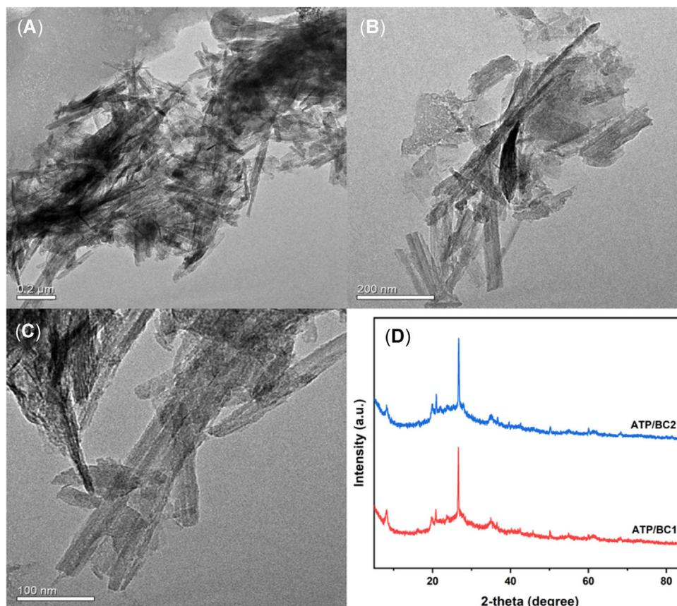
**FIGURE 2:** (A–C) Transmission electron microscopy (TEM) photograph and (D) X-ray diffractometer (XRD) spectrogram of attapulgite/biochar (ATP/BC) composites.
