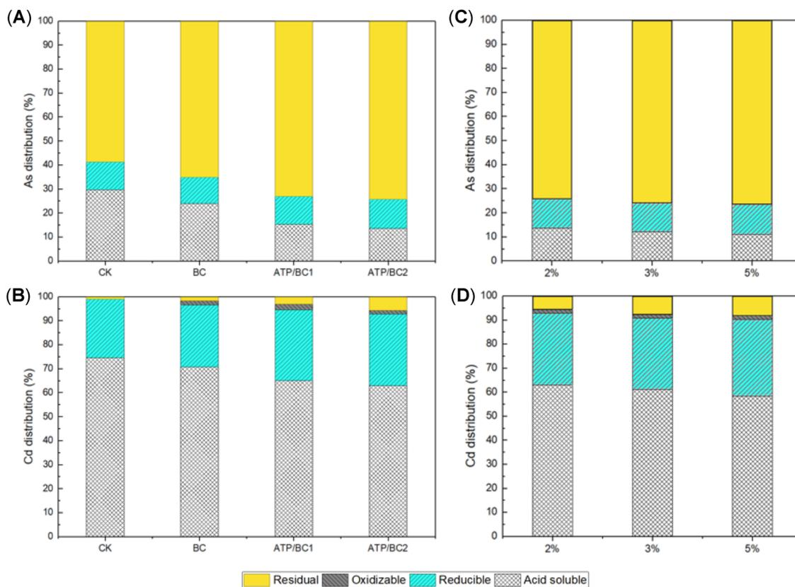
**FIGURE 5:** Fractions of arsenic (As) and cadmium (Cd) in sediment determined by Community Bureau of Reference sequential extraction after treatment with different biochars: (A) fraction of As, (B) fraction of Cd. Effect of addition amount on fraction of As and Cd in sediment determined by Community Bureau of Reference sequential extraction after treatment with attapulgite/biochar composites (ATP/BC1 and -2): (C) fraction of As, (D) fraction of Cd.
