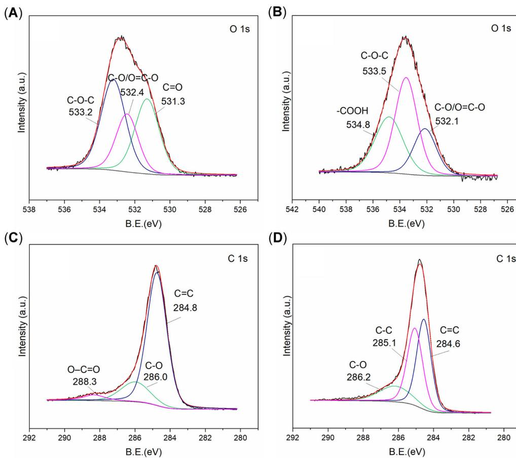
**FIGURE 3:** X-ray photoelectron spectroscopic high-resolution spectra of original biochar (A and C) and biochar/attapulgite composites (B and D). B.E. = binding energy.
