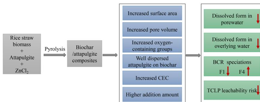
**FIGURE 7:** Possible immobilization mechanism of heavy metals in sediment by biochar/attapulgite composites. F1 and F4 are the acid-soluble fraction and the residual fraction in the solid phase of the sediment, respectively. CEC = cation exchange capacity; BCR = Community Bureau of Reference; TCLP = toxicity characteristic leaching procedure.
