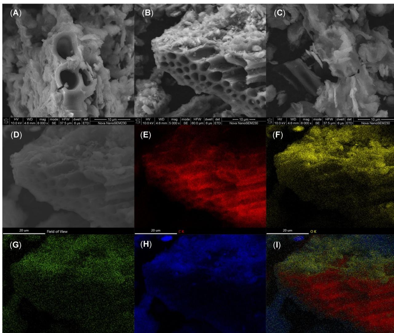
**FIGURE 1** Scanning electron microscopy (SEM) photograph and energy-dispersive X-ray (EDX) mapping of biochar/attapulgite composites: (A–C) SEM photograph, (D) field of view, (E) carbon, (F) oxygen, (G) magnesium, (H) silicon, and (I) cascading image.
