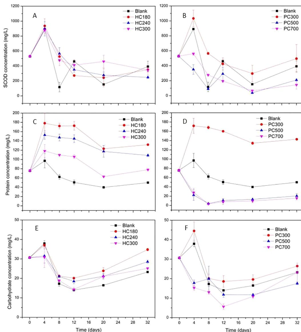
Fig. 2. Effect of hydrochar (A, C, E) and pyrochar (B, D, F) addition on soluble COD, soluble protein and soluble carbohydrate produced from the WAS anaerobic digestion.
