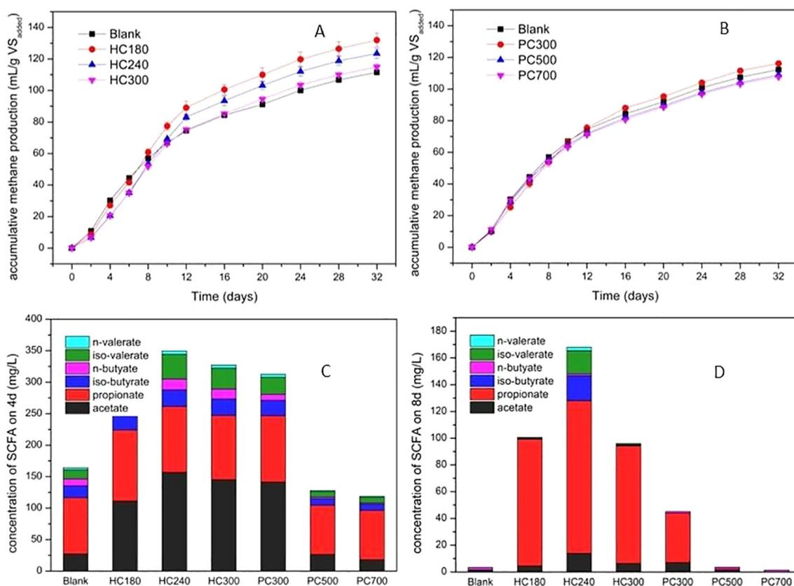
Fig. 1. The profiles of cumulative methane production with hydrochar (A) and pyrochar (B) addition; SCFA concentration and proportion on the 4th day (C) and 8th day (D).
