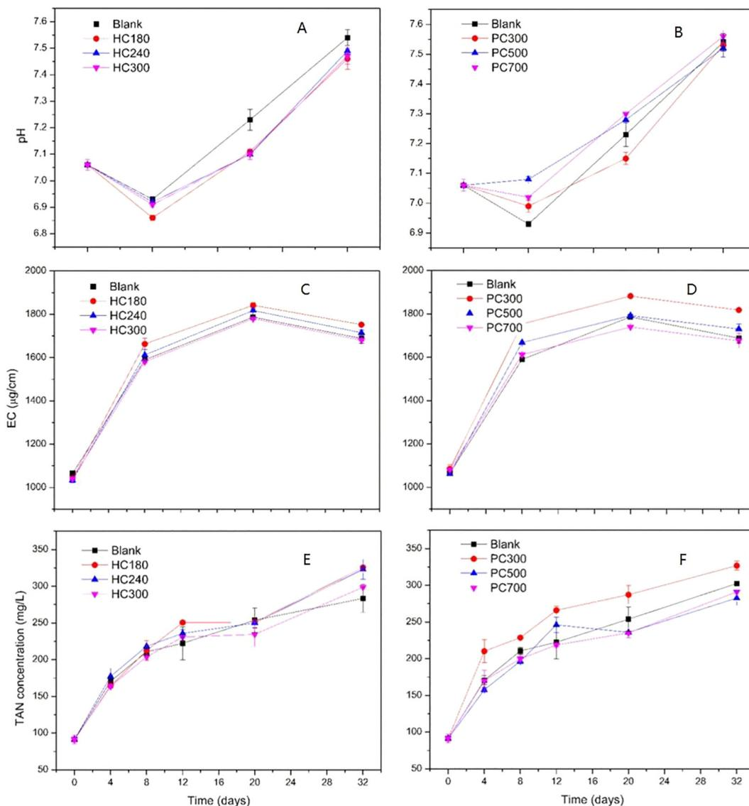
Fig. 3. Variation of pH, TAN and EC during the WAS anaerobic digestion process in presence of hydrochar (A, C, E) and pyrochar (B, D, F).
