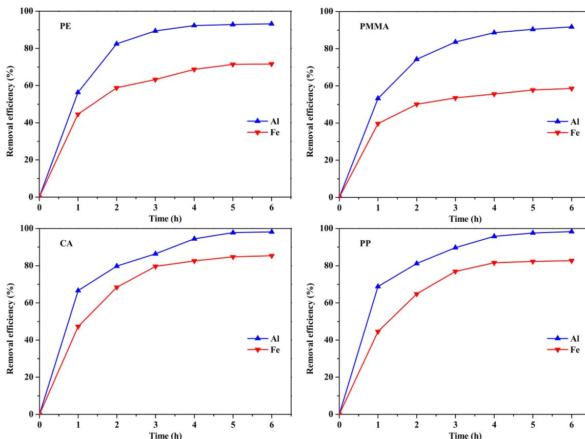
Fig. 1. Effect of Al and Fe electrode on removal of microplastics during electrocoagulation.
