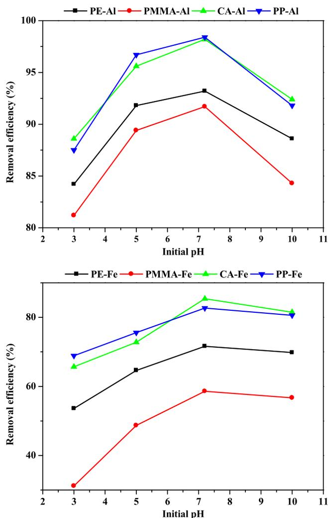
Fig. 3. Effect of initial pH on removal of microplastics during electrocoagulation.
