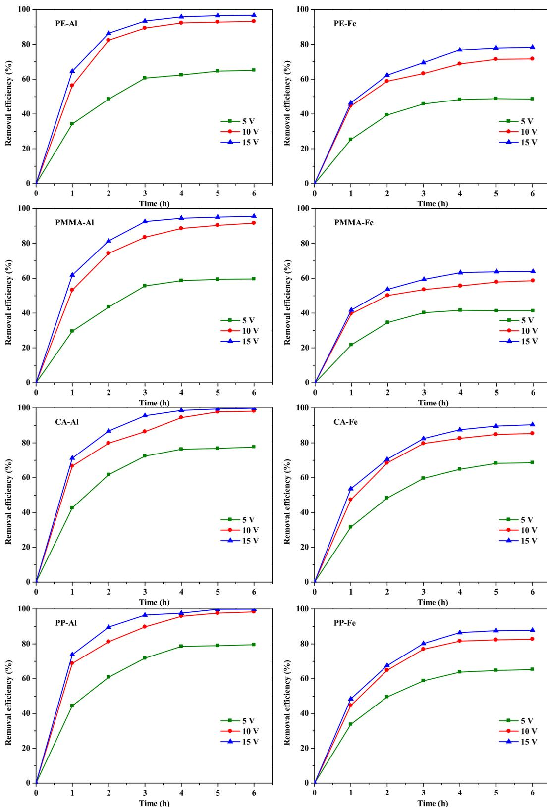
Fig. 4. Effect of different applied voltage intensity on removal of microplastics during electrocoagulation.
