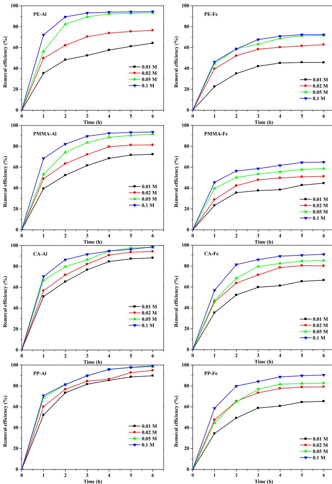
Fig. 2. Effect of different applied electrolyte concentration on removal of microplastics during electrocoagulation.
