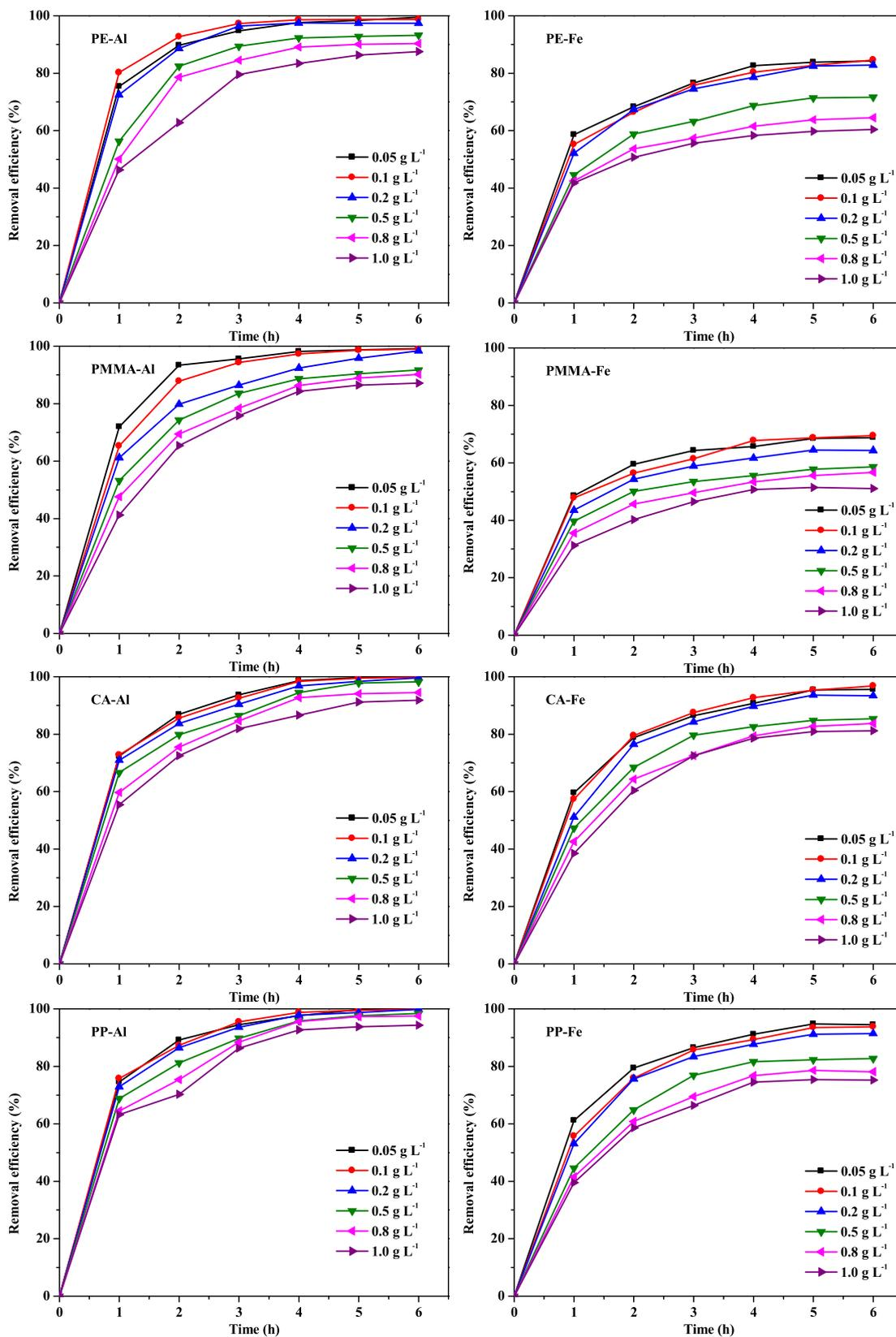
Fig. 5. Effect of microplastic concentration on removal of microplastics during electrocoagulation.
