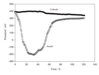
Fig. 7 – Typical evolution of redox potential the anode and the cathode for an indole-fed MFC (potentials calculated vs. SHE).
