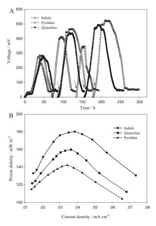
Fig. 3 – (A) Electricity generation from N-heterocyclic compounds (pyridine, quinoline and indole) using a mixed bacterial culture at a fixed resistance of  $1000 \Omega$ . (B) Power generation as a function of current density for MFCs using external resistors of  $50 \Omega$  to  $5000 \Omega$ . The arrows show the time of anode solution replacement with a different concentration ( $20 \text{ mg L}^{-1}$ ,  $60 \text{ mg L}^{-1}$ ,  $120 \text{ mg L}^{-1}$ ) of fresh medium solution.
