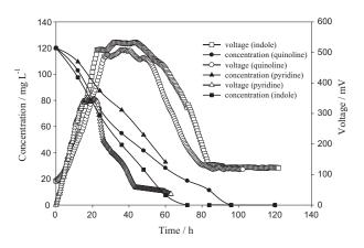
Fig. 4 – Electricity voltage output and degradation of pyridine, quinoline and indole as the sole fuel in the MFCs at the same initial concentration of  $120 \text{ mg L}^{-1}$ .
