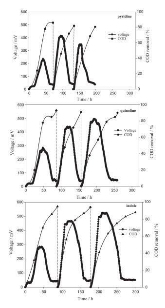
Fig. 6 – Electricity production and COD removal rates using pyridine, quinoline, and indole as the sole fuel.
