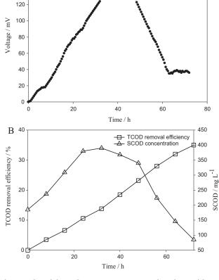
Fig. 2 – Electricity voltage output over testing time with 1000  $\Omega$  load (A) and TCOD removal efficiency as well as corresponding SCOD of sludge supernatant within MFC (B) under steady operation.
