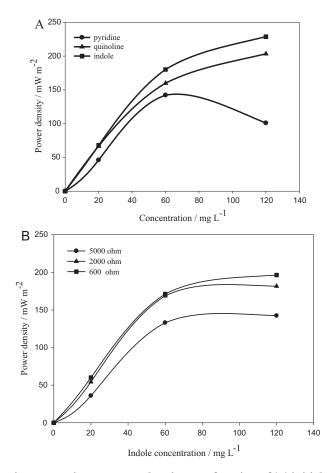
Fig. 5 – Maximum power density as a function of (A) initial various substrate concentration using a  $1000 \Omega$  resistance and (B) initial indole concentration using different resistors.
