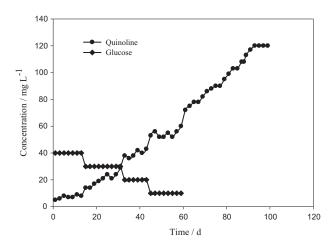
Fig. 1 – Dosing quantity of glucose and quinoline during the acclimation period of anaerobic sludge.
