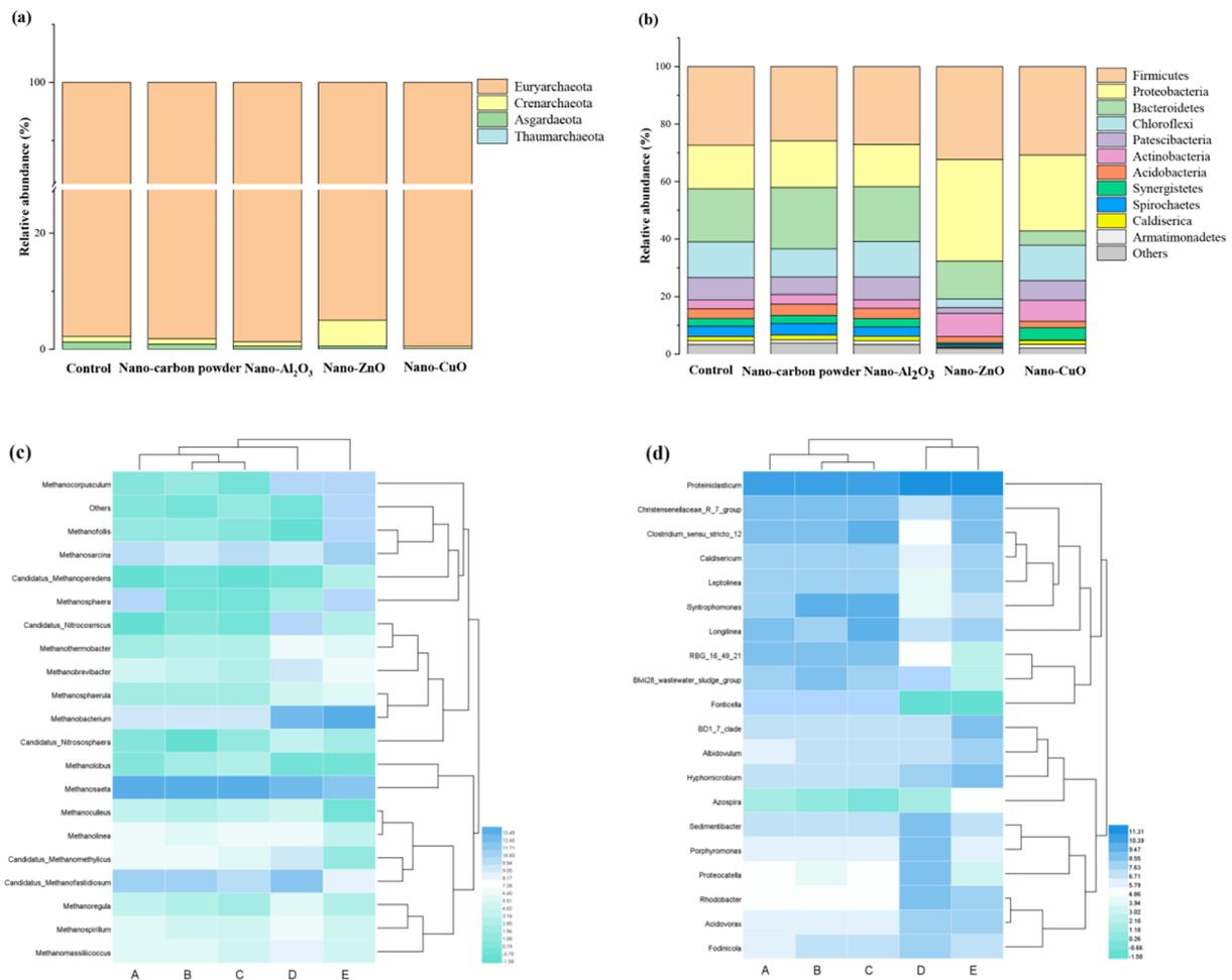
**Fig. 4.** Archaeal (a) and bacterial (b) community structure at phylum level of sludge in different reactors. Heat map demonstrated the evolution of archaea (c) and top 20 bacteria (d) at genus level in five reactors during AD. The color intensity showed the relative abundance of each genus as the color key indicated at the bottom right.
