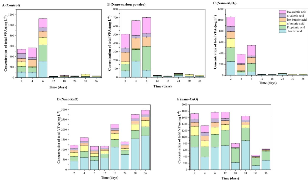
Fig. 3. Changes of total VFAs during AD in different reactors.
