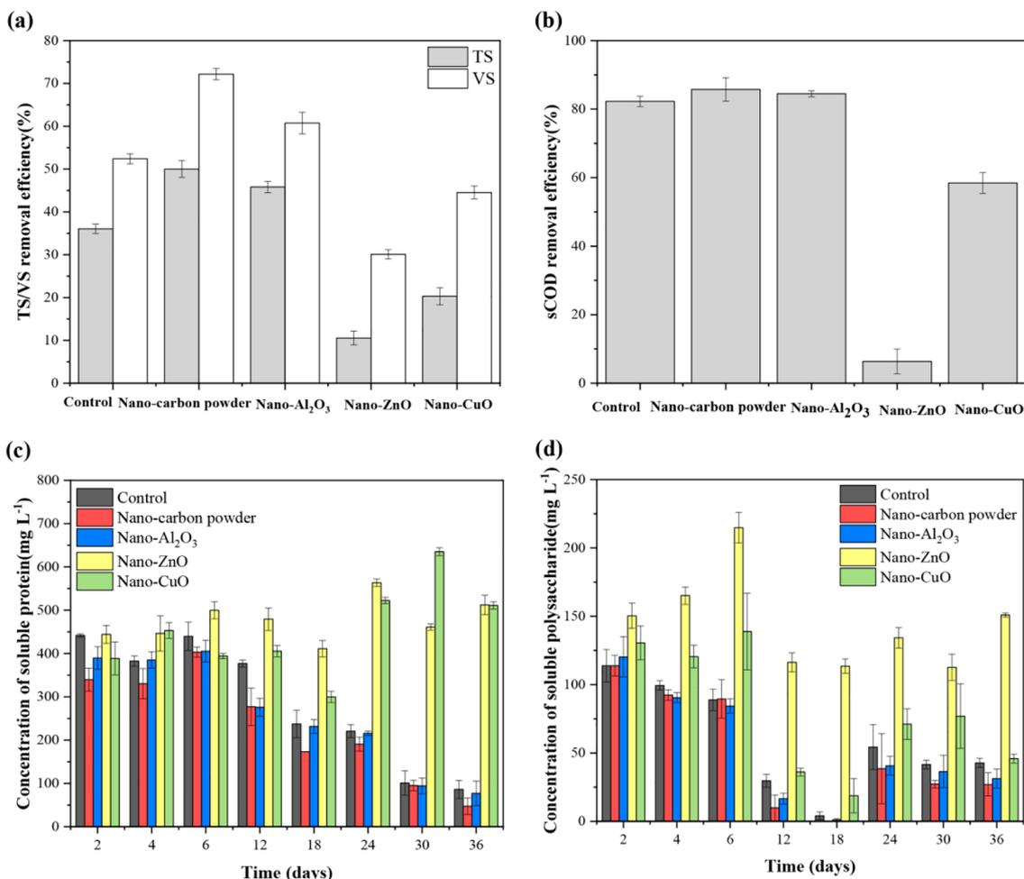
Fig. 2. TS/VS removal efficiency (a) and sCOD removal efficiency (b) of sludge in different reactors after experiments. Changes of soluble protein (c) and soluble polysaccharide (d) during AD in different reactors.
